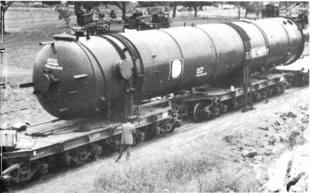
^ A huge pressure vessel makes an impressive out-of-gauge loading sight.
