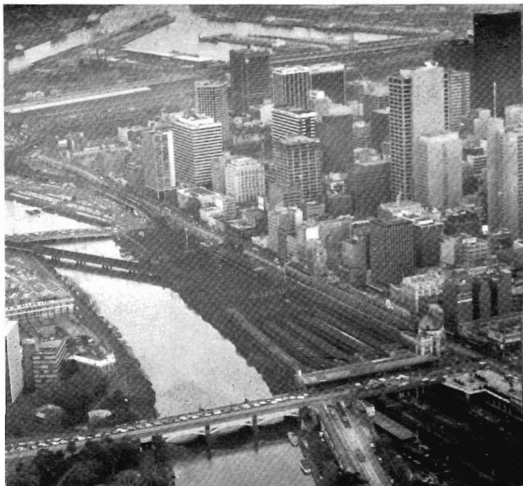
● The 11 tracks converging from Flinders Street station on to the four track viaduct to Spencer Street stand out in this picture, taken from a helicopter almost directly above Melbourne's Olympic Park sports complex.
